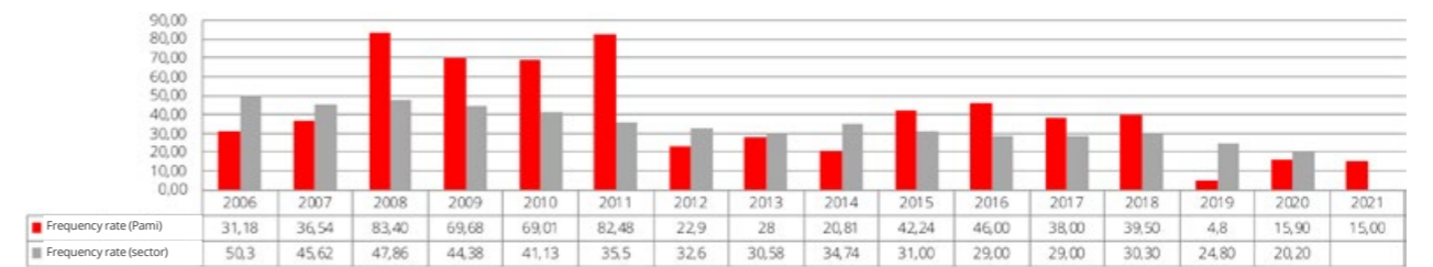
Figure 9.5 Time lost due to work accidents – Frequency rate (number of accidents x 1,000,000 / hours worked)
